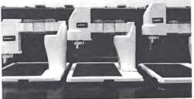
The picture to the left showcases android phones as well as other models that no current pincode breaker can get into, due to their limited interface and lack of USB OTG. Susteen's Burner Breaker can access these phones by pinpointing the location of each number and manually pressing it. Our software can go through thousands of codes and allows access to these locked phones for the first time.
